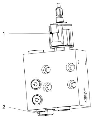
Figure 4-12 Lower lifting cylinder control valves
