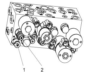
1. Pressure measuring joint 2. System main overflow valve
