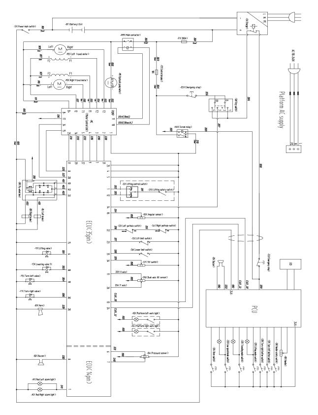
Figure 3-8 ZS1930DC Electrical schematic
