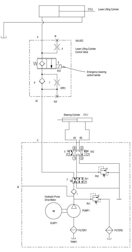
Fig.4-24 ZS1530DC Series Hydraulic schematics
