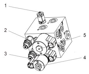
Figure 4-9 Electric driven platform control valves
