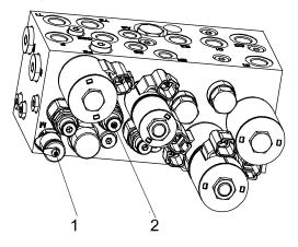
1.Pressure measuring joint 2. lifting relief valve
