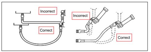
Figure 4-3 Proper bending radius
