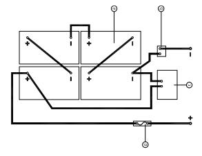
Figure 2-6 ZS4555/ZS4045/ZS3246/ZS2646/ZS2632/ZS2032/ZS1932/ZS1930 Series Battery
