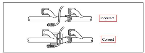
Figure 4-7 Prevent friction between parts
