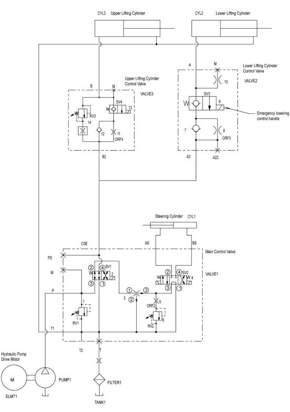
Fig. 4-21 ZS4555/ZS4045/ZS3246(DC/AC) Series Hydraulic schematics
