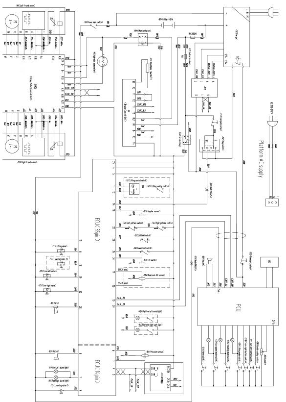
Figure 3-21 ZS1930AC-Li /ZS1932ACW-Li Electrical schematic
