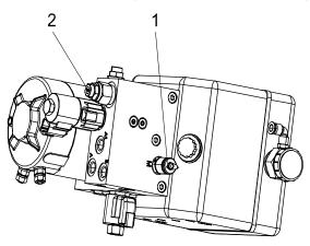
1. Pressure measuring joint 2. steering relief valve
