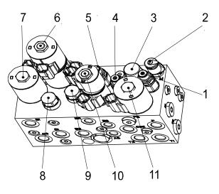
Figure 4-8 Hydraulic driven platform control valves
