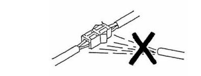
Figure 2-3 DO NOT spray water at the joint
