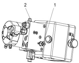
1. Pressure measuring joint 2. lifting relief valve
