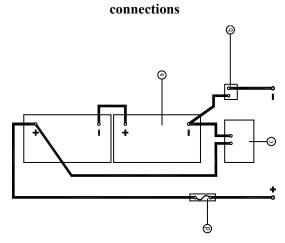
Figure 2-7 ZS1930DCS/ZS1530DC Battery connections
