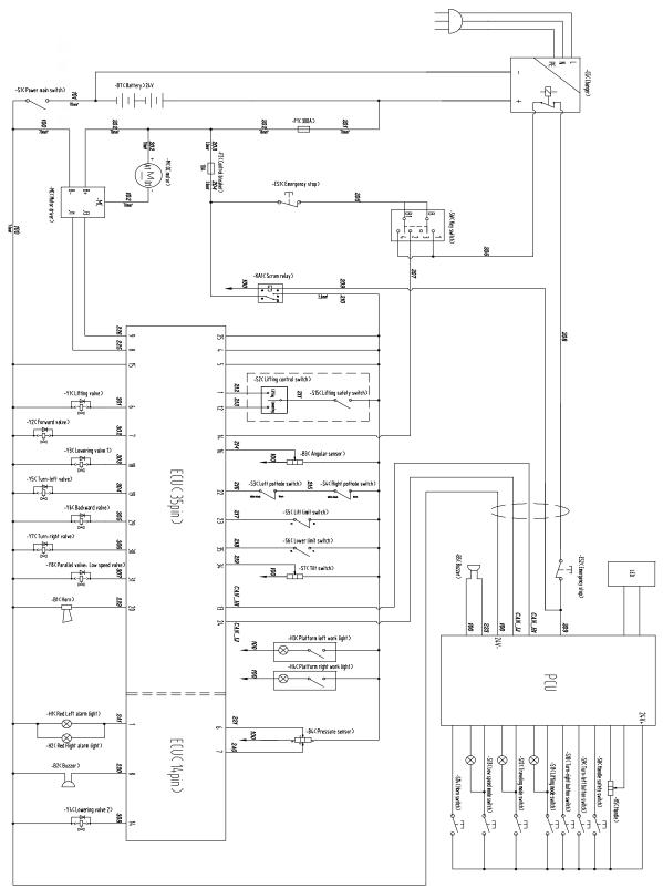
Figure 3-3 ZS4555HD/ZS4045HD/ZS3246HD Electrical schematic
