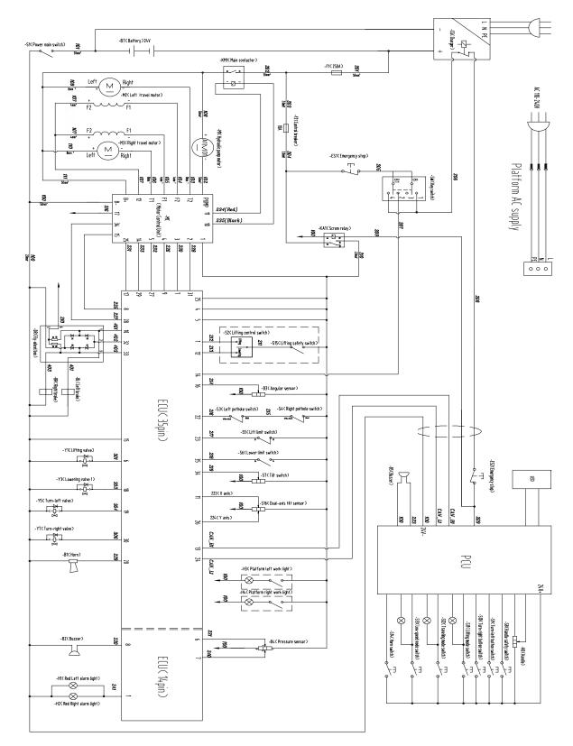
Figure 3-7 ZS2646DC/ZS2632DC/ZS2032DC Electrical schematic
