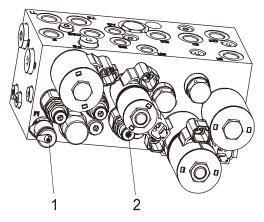
1. Pressure measuring joint 2. steering relief valve
