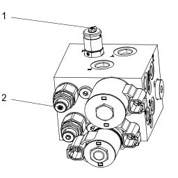
1. Pressure measuring joint 2. lifting relief valve
