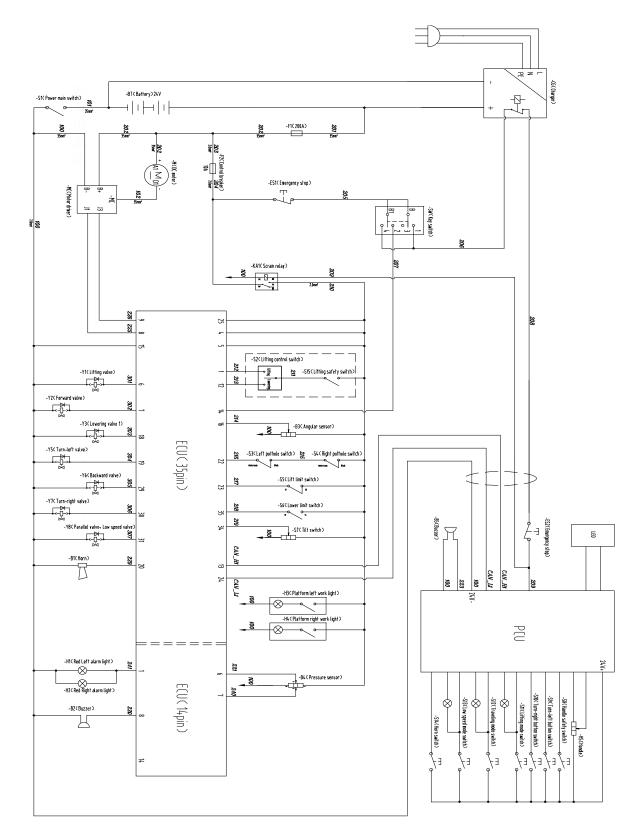
Figure 3-5 ZS1930HD Electrical schematic
