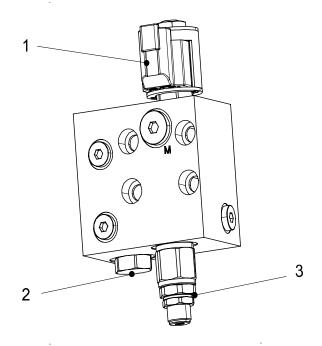
Figure 4-11 Upper lifting cylinder control valves
