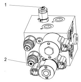
1. Pressure measuring joint 2. steering relief valve
