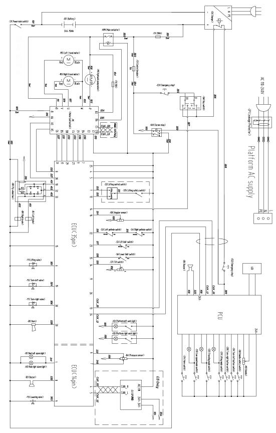
Figure 3-9 ZS1930DCS Electrical schematic
