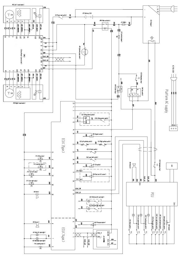
Figure 3-19 ZS1930AC/ZS1932ACW Electrical schematic
