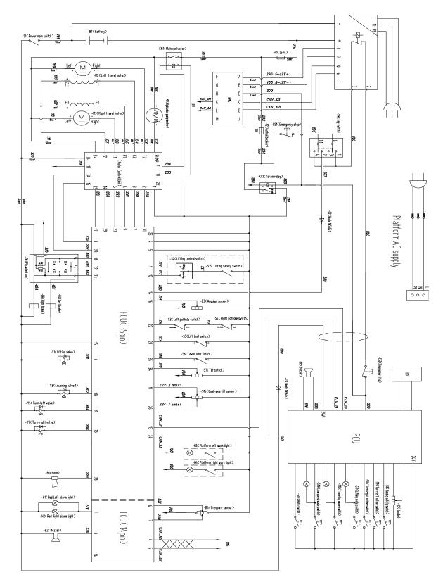
Figure 3-15 ZS2646DC-Li/ZS2632DC-Li/ZS2032DC-Li Electrical schematic
