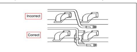
Effectively reduces abrasion between hoses and associated components.
